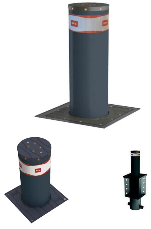
K4 equivalent anti-terrorism bollard, based on dynamic simulation carried out by accredited third-party laboratory to international standards ASTM2656:2007 M30 – PAS68:2010 7500/50/N2
